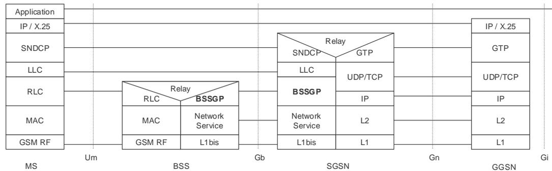
**Figure 8 GPRS Protocol Stack**
