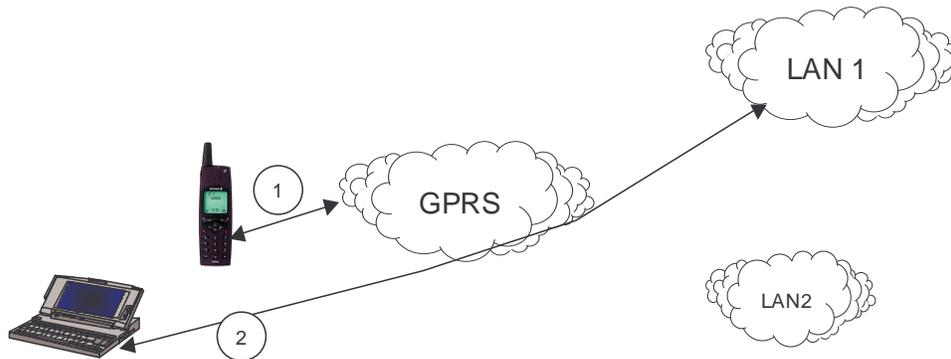
Figure 5 GPRS attach (1) and PDP context activation (2)
