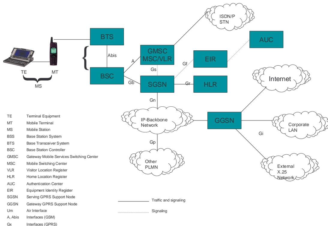
**Figure 3 GPRS Logical Architecture**
