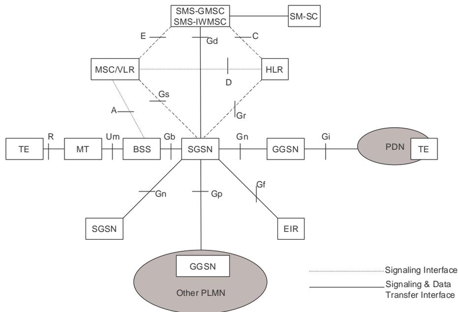
**Figure 12 GPRS Logical Architecture**
